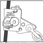
**6.** Check locking action by pulling down on rope grab handle.
