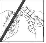
Depress the button on the safety locking pin and remove from main
