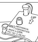
5. Make sure that locking pin balls appear on outside of main assembly and the direction arrow on the housing is pointing up. **3.** Place rope grab on rope with plastic roller pointing up.
