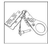
2. Swing cam and lever assembly up and open.
