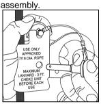
**4.** Close assembly, align holes and reinsert safety locking pin.
