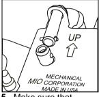
5. Make sure that locking pin balls appear on outside of main assembly and the direction arrow on the housing is pointing up.
