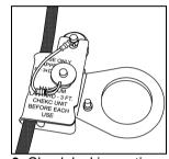
**6.** Check locking action by pulling down on rope grab handle.
