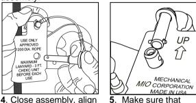
5. Make sure that locking pin balls appear on outside of main assembly and the direction arrow on the housing is pointing up.
